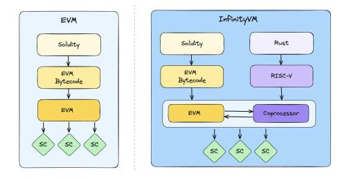
Figure 2: InfinityVM enshrines coprocessing alongside the EVM
