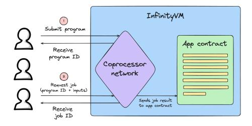
Figure 8: System architecture with an enshrined coprocessor receiving requests
