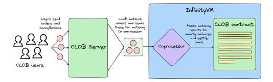
Figure 11: How the CLOB application works: running compute offchain and running state transitions through the coprocessor
